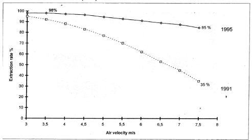
Average curve based on following standards : SAE , DOS , Atmospheric Air Test carried out by SINTEF INSTITUTE, 1995
